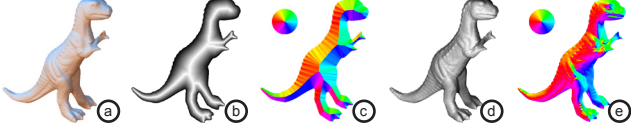
Figure 3. Objects that are convex or composed of convex parts (a) exhibit a strong correlation between silhouette-based features like relative distance (b) or direction to the silhouette (c) and out-of-plane (d) and in-plane components (e) of their surface normals.
