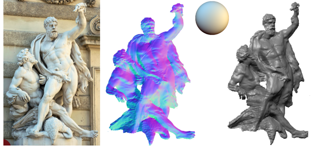
Figure 1. Qualitative results for shape and reflectance estimation from a single image: input image [30], estimated normals and reflectance map from our method, and novel view (from left to right).
